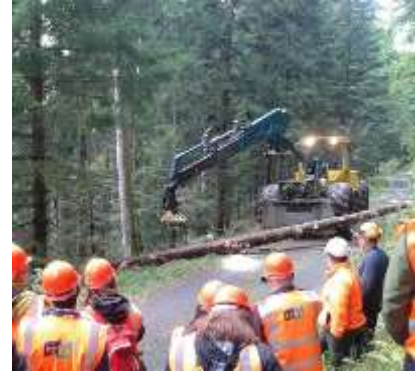
Long logs were hauled to the road side with a grapple skidder also equipped with a cable
