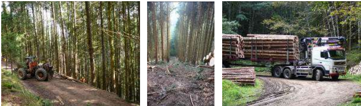
The rest of the site was harvested with motor-manual equipment and logs were hauled on the roadside with a skidder
