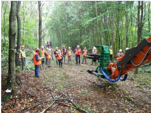
The shear heads C360 (Jacquier's red) and S350 (Seve's green) mounted on excavators were demonstrated on site in an oak stand
