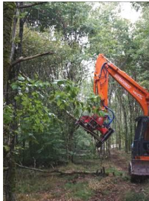
The shear heads C360 (Jacquier's red) and S350 (Seve's green) mounted on excavators were demonstrated on site in an oak stand
