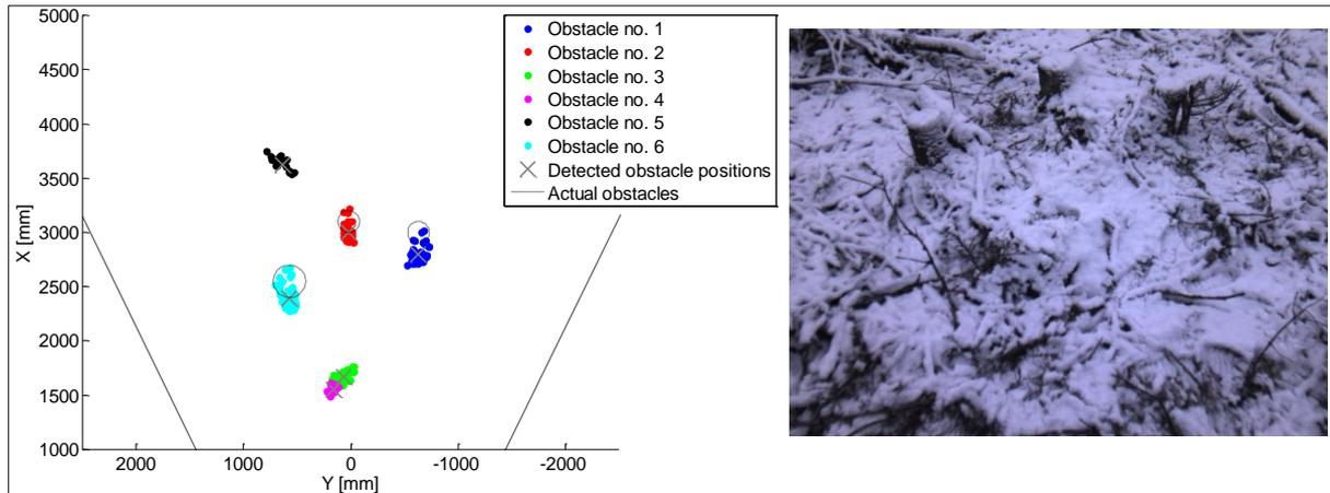
The post-processing algorithm uses ~3 seconds on an office laptop @ 2.7 GHz to process each snapshot of around 5x5 metres. This gives a maximum advancement speed of 1.7 m/s, (not accounting for time delay of the actions taken by the machine given the identified obstacles) which is sufficient for many existing machines.
