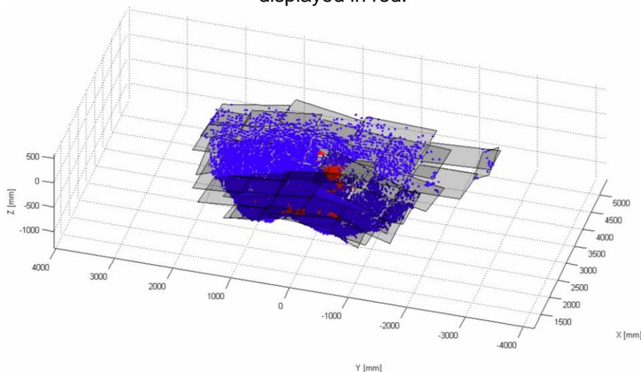
These remaining pixel clusters were considered as obstacles whereby the centre coordinate of the cluster was marked. A comparison with real measurements was conducted, and the accuracy was calculated.
