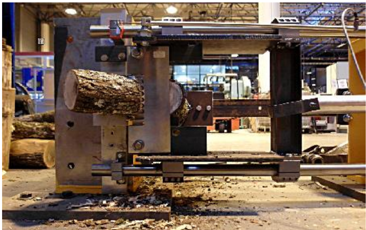
Figure 6: Delimiting with an innovative ribbed knife. The branch bends a lot before cutting.
