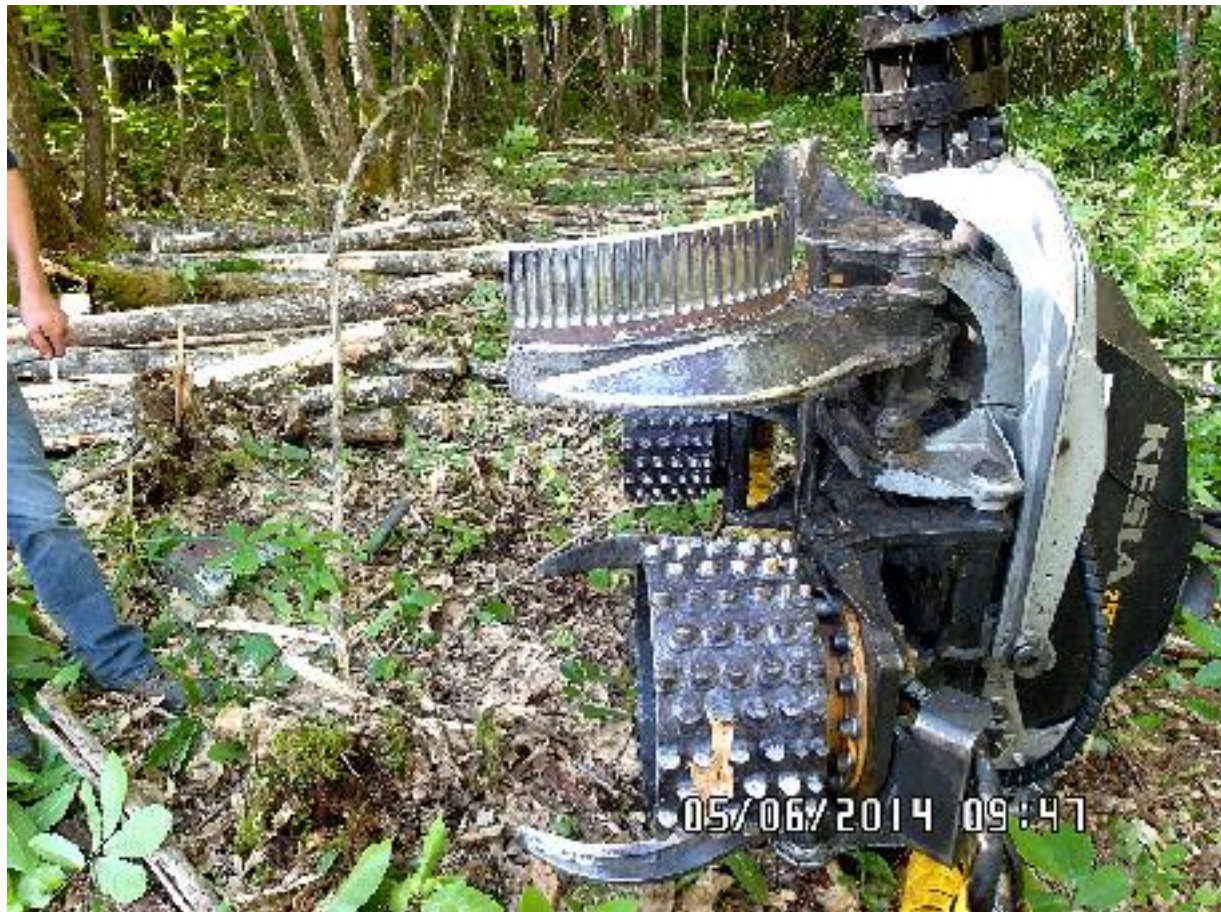
Figure 9: A prototype ribbed knife replacing the top classical knife on a Kesla 25RH head.
