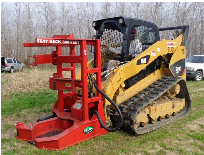
Figure 1. Shear-head mounted on skid steer.
